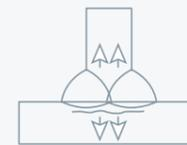
Stresses in the direction of plate thickness caused by welding
